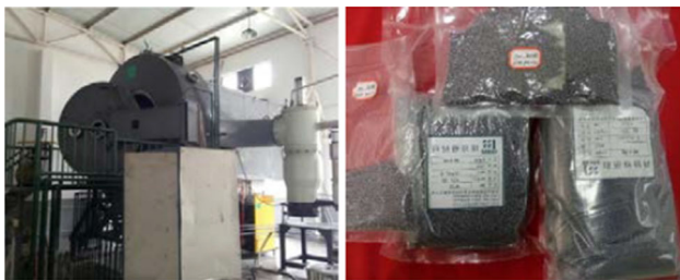
Fig. 21 Beryllium pebble fabrication facility and product
