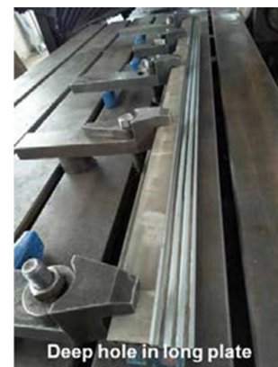
Fig. 33 Deep hole drilling for Ø6 mm holes in 2 m long plate and its destructive inspection
