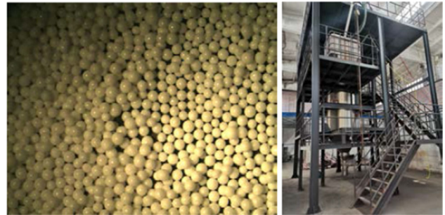
Fig. 22 Lithium silicate pebble and its new fabrication facility
