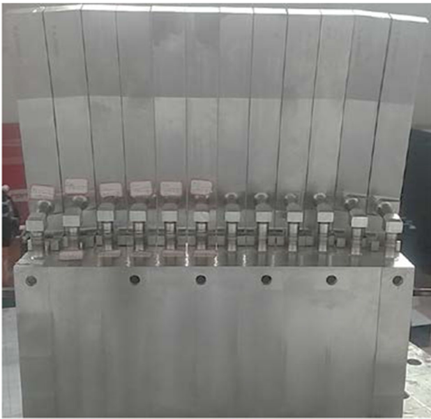
Fig. 5 A dummy FW assembly showing the stainless-steel fingers mounted to a central beam with pipe connections
