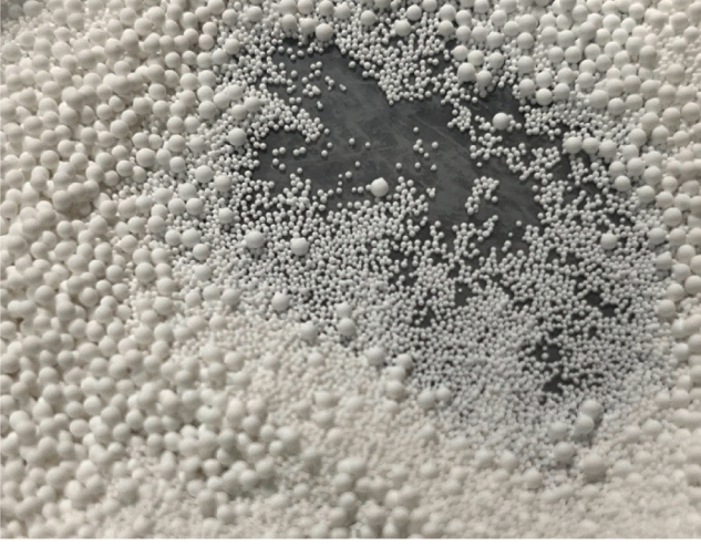
Fig. 6. Comparison of two sizes of alumina particles.
